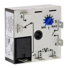
ProSense off-delay relay timer, 1 to 100 minutes timing range, 24 VAC/VDC operating voltage, 10A contact rating, (1) SPDT timed relay output(s), surface mount, 1/4in male quick-connect terminal.
