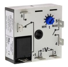
ProSense off-delay relay timer, 0.1 to 10 minutes timing range, 120 VAC/VDC operating voltage, 10A contact rating, (1) SPDT timed relay output(s), surface mount, 1/4in male quick-connect terminal.
