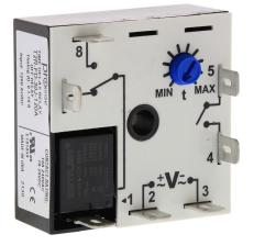
ProSense off-delay relay timer, 0.1 to 10 seconds timing range, 120 VAC/VDC operating voltage, 10A contact rating, (1) SPDT timed relay output(s), surface mount, 1/4in male quick-connect terminal.
