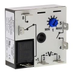
ProSense off-delay relay timer, 0.1 to 10 seconds timing range, 24 VAC/VDC operating voltage, 10A contact rating, (1) SPDT timed relay output(s), surface mount, 1/4in male quick-connect terminal.
