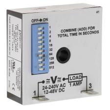
ProSense on-delay inline relay timer, 1 to 1,023 seconds selectable timing range, 24-240 VAC and 12-48 VDC operating voltage, 1A contact rating, (1) SPNO timed solid state relay output(s), surface mount, 1/4in male quick-connect terminal.
