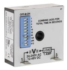
ProSense on-delay inline relay timer, 1 to 1,023 seconds selectable timing range, 24-240 VAC and 12-48 VDC operating voltage, 1A contact rating, (1) SPNO timed solid state relay output(s), surface mount, 1/4in male quick-connect terminal.
