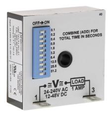
ProSense on-delay inline relay timer, 0.1 to 102.3 seconds selectable timing range, 24-240 VAC and 12-48 VDC operating voltage, 1A contact rating, (1) SPNO timed solid state relay output(s), surface mount, 1/4in male quick-connect terminal.
