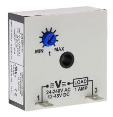
ProSense on-delay inline relay timer, 1 to 100 minutes timing range, 24-240 VAC and 12-48 VDC operating voltage, 1A contact rating, (1) SPNO timed solid state relay output(s), surface mount, 1/4in male quick-connect terminal.
