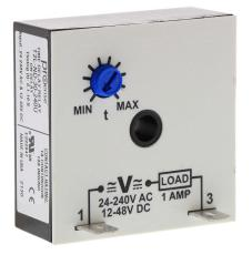
ProSense on-delay inline relay timer, 0.1 to 10 seconds timing range, 24-240 VAC and 12-48 VDC operating voltage, 1A contact rating, (1) SPNO timed solid state relay output(s), surface mount, 1/4in male quick-connect terminal.
