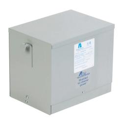
ACME general purpose transformer, encapsulated core, 6 kVA, 3-phase, 600 VAC Delta primary, 480Y/277 VAC secondary, 60 Hz, electrostatic shield, NEMA 3R, wall mount.
