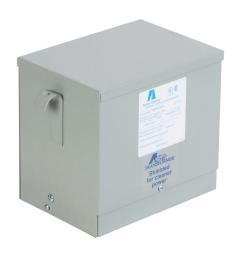
ACME general purpose transformer, encapsulated core, 3 kVA, 3-phase, 600 VAC Delta primary, 480Y/277 VAC secondary, 60 Hz, electrostatic shield, NEMA 3R, wall mount.
