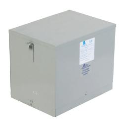
ACME general purpose transformer, encapsulated core, 9 kVA, 3-phase, 600 VAC Delta primary, 208Y/120 VAC secondary, 60 Hz, electrostatic shield, NEMA 3R, wall mount.
