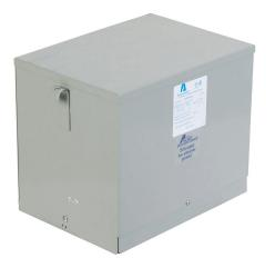
ACME general purpose transformer, encapsulated core, 9 kVA, 3-phase, 600 VAC Delta primary, 208Y/120 VAC secondary, 60 Hz, electrostatic shield, NEMA 3R, wall mount.
