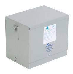
ACME general purpose transformer, encapsulated core, 6 kVA, 3-phase, 600 VAC Delta primary, 208Y/120 VAC secondary, 60 Hz, electrostatic shield, NEMA 3R, wall mount.
