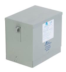
ACME general purpose transformer, encapsulated core, 3 kVA, 3-phase, 600 VAC Delta primary, 208Y/120 VAC secondary, 60 Hz, electrostatic shield, NEMA 3R, wall mount.
