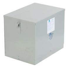
ACME general purpose transformer, encapsulated core, 9 kVA, 3-phase, 480 VAC Delta primary, 240/120 VAC Delta (center tap) secondary, 60 Hz, electrostatic shield, NEMA 3R, wall mount.
