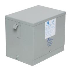
ACME general purpose transformer, encapsulated core, 6 kVA, 3-phase, 480 VAC Delta primary, 240/120 VAC Delta (center tap) secondary, 60 Hz, electrostatic shield, NEMA 3R, wall mount.
