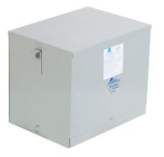
ACME general purpose transformer, encapsulated core, 9 kVA, 3-phase, 480 VAC Delta primary, 208Y/120 VAC secondary, 60 Hz, electrostatic shield, NEMA 3R, wall mount.
