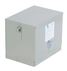
ACME general purpose transformer, encapsulated core, 6 kVA, 3-phase, 480 VAC Delta primary, 208Y/120 VAC secondary, 60 Hz, electrostatic shield, NEMA 3R, wall mount.
