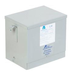
ACME general purpose transformer, encapsulated core, 3 kVA, 3-phase, 480 VAC Delta primary, 208Y/120 VAC secondary, 60 Hz, electrostatic shield, NEMA 3R, wall mount.
