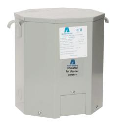
ACME general purpose transformer, encapsulated core, 7.5 kVA, 1-phase, 120/208/240/277 VAC primary, 120/240 VAC secondary, 60 Hz, electrostatic shield, NEMA 3R, wall mount.
