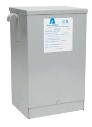
ACME general purpose transformer, encapsulated core, 5 kVA, 1-phase, 120/208/240/277 VAC primary, 120/240 VAC secondary, 60 Hz, electrostatic shield, NEMA 3R, wall mount.
