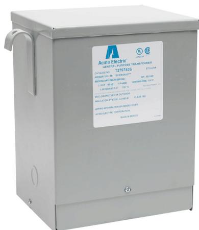
ACME general purpose transformer, encapsulated core, 3 kVA, 1-phase, 120/208/240/277 VAC primary, 120/240 VAC secondary, 60 Hz, electrostatic shield, NEMA 3R, wall mount.
