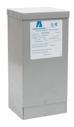
ACME general purpose transformer, encapsulated core, 2 kVA, 1-phase, 120/208/240/277 VAC primary, 120/240 VAC secondary, 60 Hz, electrostatic shield, NEMA 3R, wall mount.
