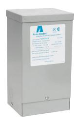
ACME general purpose transformer, encapsulated core, 1.5 kVA, 1-phase, 120/208/240/277 VAC primary, 120/240 VAC secondary, 60 Hz, electrostatic shield, NEMA 3R, wall mount.
