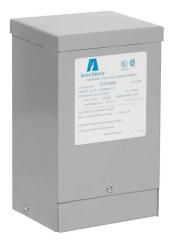
ACME general purpose transformer, encapsulated core, 1 kVA, 1-phase, 120/208/240/277 VAC primary, 120/240 VAC secondary, 60 Hz, electrostatic shield, NEMA 3R, wall mount.
