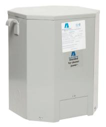
ACME general purpose transformer, encapsulated core, 15 kVA, 1-phase, 600 VAC primary, 120/240 VAC secondary, 60 Hz, electrostatic shield, NEMA 3R, wall mount.
