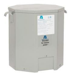
ACME general purpose transformer, encapsulated core, 10 kVA, 1-phase, 600 VAC primary, 120/240 VAC secondary, 60 Hz, electrostatic shield, NEMA 3R, wall mount.
