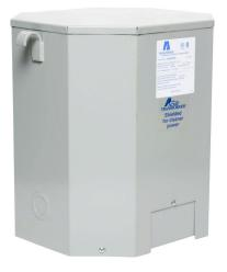
ACME general purpose transformer, encapsulated core, 25 kVA, 1-phase, 240/480 VAC primary, 120/240 VAC secondary, 60 Hz, electrostatic shield, NEMA 3R, wall mount.
