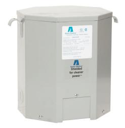
ACME general purpose transformer, encapsulated core, 10 kVA, 1-phase, 240/480 VAC primary, 120/240 VAC secondary, 60 Hz, electrostatic shield, NEMA 3R, wall mount.
