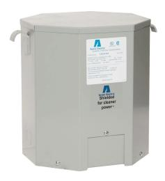
ACME general purpose transformer, encapsulated core, 7.5 kVA, 1-phase, 240/480 VAC primary, 120/240 VAC secondary, 60 Hz, electrostatic shield, NEMA 3R, wall mount.
