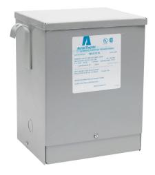
ACME general purpose transformer, encapsulated core, 3 kVA, 1-phase, 600 VAC primary, 120/240 VAC secondary, 60 Hz, electrostatic shield, NEMA 3R, wall mount.
