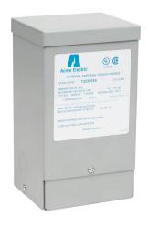
ACME general purpose transformer, encapsulated core, 750 VA, 1-phase, 600 VAC primary, 120/240 VAC secondary, 50/60 Hz, electrostatic shield, NEMA 3R, wall mount.
