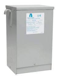
ACME general purpose transformer, encapsulated core, 5 kVA, 1-phase, 240/480 VAC primary, 120/240 VAC secondary, 60 Hz, electrostatic shield, NEMA 3R, wall mount.
