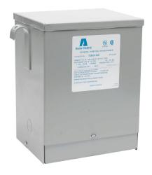
ACME general purpose transformer, encapsulated core, 3 kVA, 1-phase, 240/480 VAC primary, 120/240 VAC secondary, 60 Hz, electrostatic shield, NEMA 3R, wall mount.
