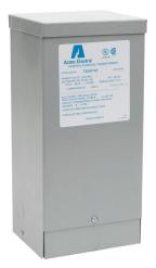
ACME general purpose transformer, encapsulated core, 2 kVA, 1-phase, 240/480 VAC primary, 120/240 VAC secondary, 60 Hz, electrostatic shield, NEMA 3R, wall mount.
