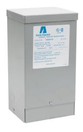
ACME general purpose transformer, encapsulated core, 1.5 kVA, 1-phase, 240/480 VAC primary, 120/240 VAC secondary, 60 Hz, electrostatic shield, NEMA 3R, wall mount.
