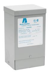
ACME general purpose transformer, encapsulated core, 750 VA, 1-phase, 240/480 VAC primary, 120/240 VAC secondary, 50/60 Hz, electrostatic shield, NEMA 3R, wall mount.
