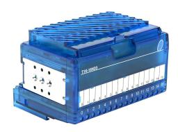
Terminator discrete input module, 16-point, 12-24 VDC, sinking/sourcing, 4 isolated common(s), 4 point(s) per common. Requires T1K-16B or T1K-16B-1 terminal base.
