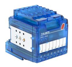
Terminator relay output module, 8-point, 6-24 VDC/6-240 VAC, (8) Form A, 2 isolated common(s), 4 point(s) per common, 2A/point, 8A/common. Requires T1K-08B or T1K-08B-1 terminal base.
