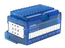
Terminator relay output module, 8-point, 6-24 VDC/6-240 VAC, (8) Form A, 8 isolated common(s), 1 point(s) per common, 7A/point. Requires T1K-16B or T1K-16B-1 terminal base.
