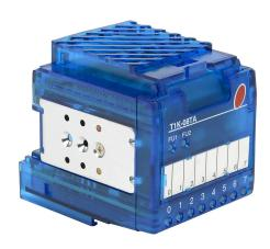
Terminator discrete output module, 8-point, 24-240 VAC, 2 isolated common(s), 4 point(s) per common, 1A/point, 4A/common. Requires T1K-08B or T1K-08B-1 terminal base.
