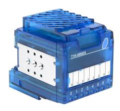
Terminator discrete input module, 8-point, 12-24 VDC, sinking/sourcing, 2 isolated common(s), 4 point(s) per common. Requires T1K-08B or T1K-08B-1 terminal base.
