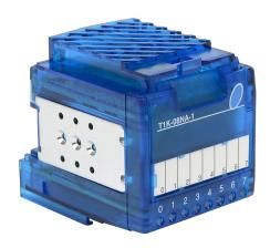
Terminator discrete input module, 8-point, 120 VAC, 2 isolated common(s), 4 point(s) per common. Requires T1K-08B or T1K-08B-1 terminal base.
