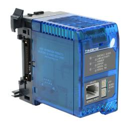
Terminator Ethernet base controller, (1) Ethernet 10/100Base-T (RJ45) port(s), Do-more Ethernet remote I/O, Modbus TCP/IP, TCP/IP, UDP/IP and IPX, up to 100 Mbps.
