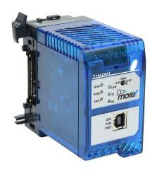
Do-more T1H CPU, 64k words ladder memory, (1) RS-232 (RJ12) and (1) USB B port(s), battery included.
