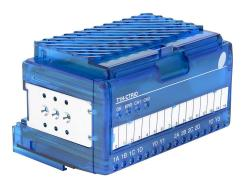
Terminator pulse combo module, 100 kHz maximum switching frequency, 8 high-speed input point(s), sinking/sourcing, single-ended encoder input(s), 4 high-speed output point(s), sinking/ sourcing, single-ended output(s).
