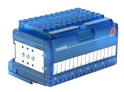
Terminator discrete output module, 8-point, 6-24 VDC, sinking and sourcing, 8 isolated common(s), 1 point(s) per common, 2A/point, 16A/module, overcurrent protection. Requires T1K-16B or T1K-16B-1 terminal base.
