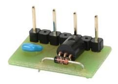
Terminator CJC sensor, replacement. For use with T1F-14THM temperature input module.
