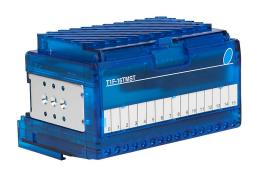
Terminator temperature input module, thermistor, 16-channel, 16-bit resolution, input thermistor type(s): 2252, 10K-AN Type 3, 10K-CP Type 2, 5K, 3K and 1.8K ohm. Requires T1K-16B or T1K-16B-1 terminal base.
