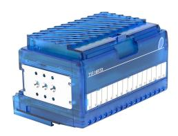
Terminator temperature input module, RTD, 16-channel, 16-bit resolution, input RTD type(s): Pt100, JPt100, Cu10, Cu25 and Pt1000. Requires T1K-16B or T1K-16B-1 terminal base.
