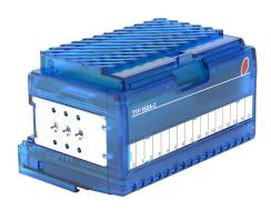
Terminator analog output module, 16-channel, voltage, 12-bit, output voltage signal range(s) of 0-5 VDC, 0-10 VDC, +/- 5 VDC and +/- 10 VDC, external 24 VDC required.
