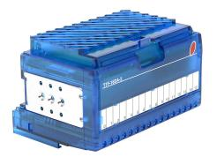
Terminator analog output module, 16-channel, voltage, 12-bit, external 24 VDC required. Requires T1K-16B or T1K-16B-1 terminal base.
